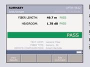
PASS/FAIL insertion loss analysis makes it easy to see whether the fiber is good – and presents the data in a clear, easy-tointerpret format.
