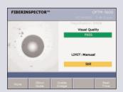
The fiber inspection camera provides a high-resolution 250x endface image of the fiber connector. Grade the image. Save the image – and show it to your customer.
