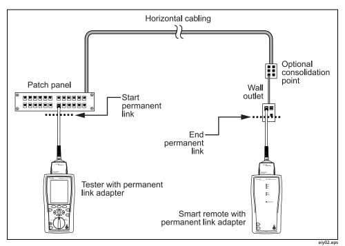
Figure 2. Connecting to a Permanent Link
