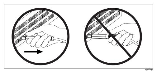
Figure 3. Disconnecting the Plug from a Jack
