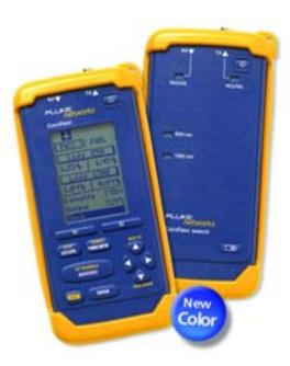
single Autotest-initiated operation. Bi-directional testing is simple too. In bi-directional mode, simply reverse Tx/Rx fibers at the patch panel or outlet when prompted and CertiFiber measures each fiber at both wavelengths in both directions – without having to swap sources and meters as with a traditional test set. CertiFiber cuts your test time by 75% over traditional techniques.
