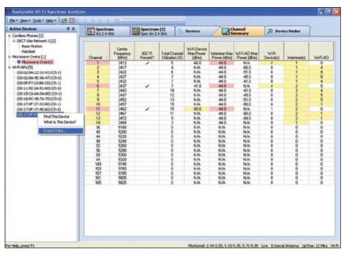
Quickly determine which channels contain 802.11 network devices, the number of interfering devices on those channels and the channel's current max power in dBm. With this information, you can quickly determine which of your channels are being impacted by interference.
