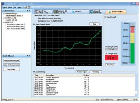
Easily locate interference in 802.11 WLANs with Device Finder. Simply click on the offending device and Device Finder will tell you its signal strength. As you move closer or farther away from the device, Device Finder's signal strength will change, allowing you to quickly narrow in on the offending device and determine its exact location.
